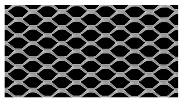
LW Pitch:25.40mmStrand Width:3.00mmSW Pitch:13.50mmThickness:0.90mmWeight:3.15 kg / m2Open Area:56%
